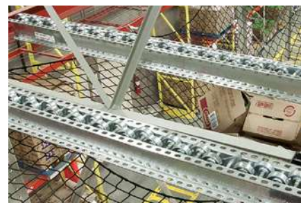
Horizontal safety netting
