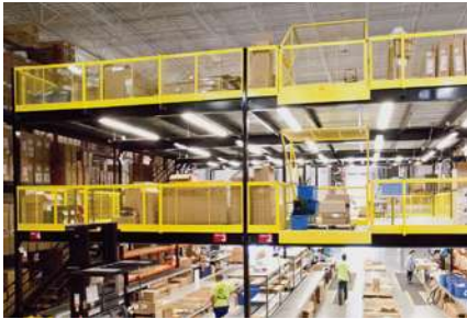
Storage platform with packing stations
